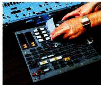
Modules may be removed individually without disconnection from cable harness.
